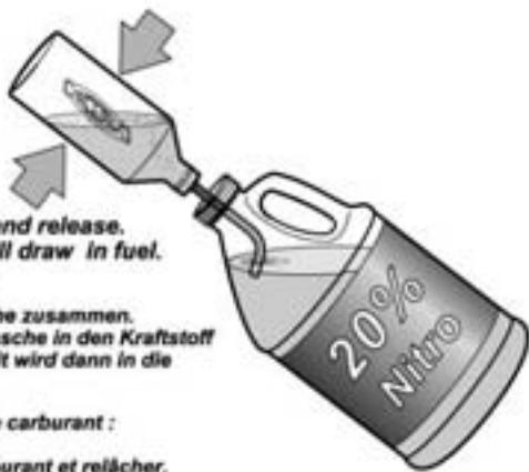
**Fill the tank completely with fuel. Use 20% Nitro content fuel only. Use good quality branded model car fuel only. Using the wrong fuel could damage your engine. Do not use Gasoline.**
