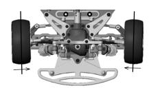
Toe-in: Easier to drive. Improves stability during acceleration.
