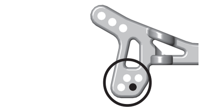
Camber link possibilities for the front tower. Standard setup shown.
